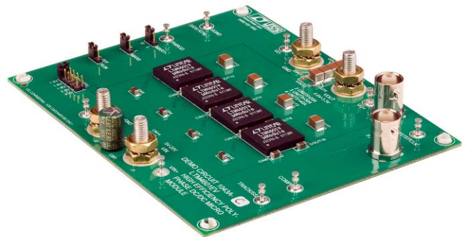
Figure 1. Four DC/DC \mu Module Regulator Systems Current Share to Regulate 1.5V at 48A with Only 2.8mm Profile and 15mm \times 15mm of Board Area. Each \mu Module Regulator Weighs Only 1.7g and Has an IC Form-Factor That Can Easily Be Used with Any Pick-and-Place Machine During Board Assembly
